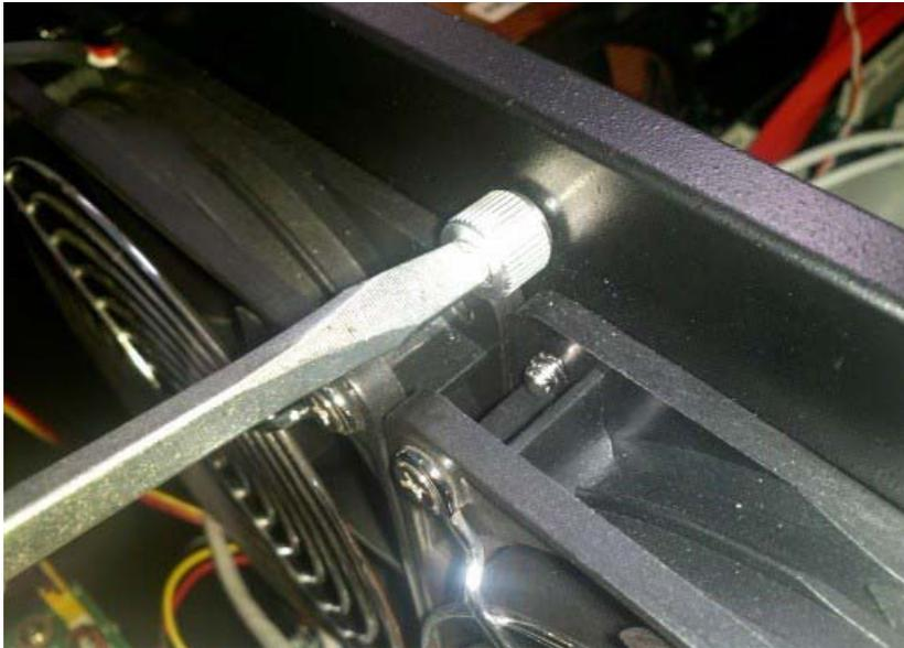
**Figure 2–4:** Fan Tray Thumb Screw
