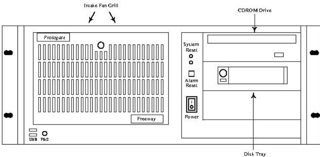
Figure 1–2: Front View of the Freeway 3414/3414R (access door not shown)
