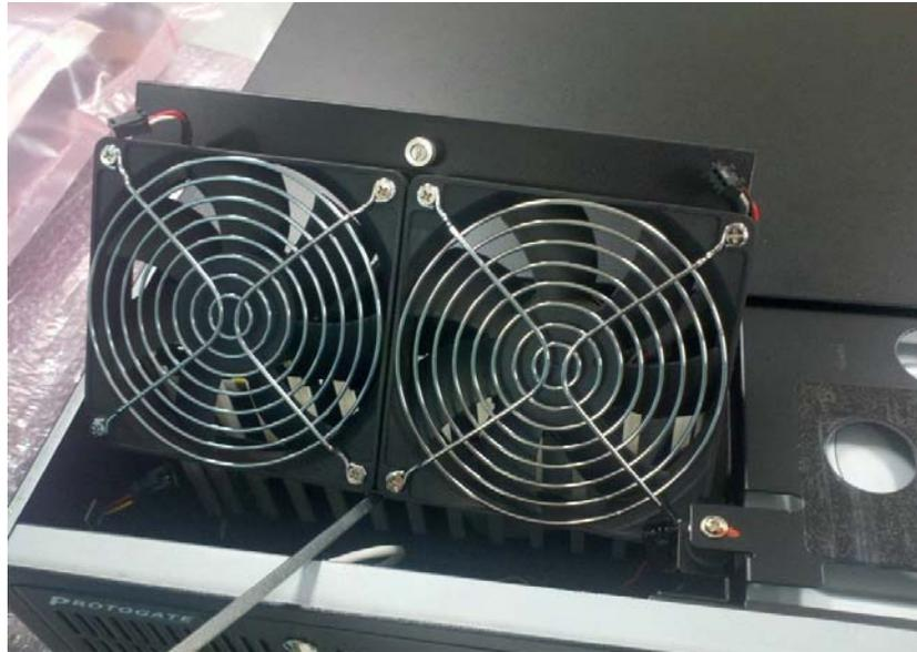
**Figure 2–5:** Fan Tray Assembly
