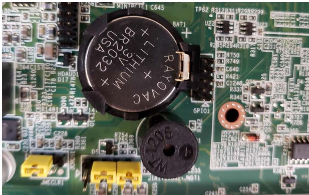
**Figure 4-5:** CPU CMOS Battery
