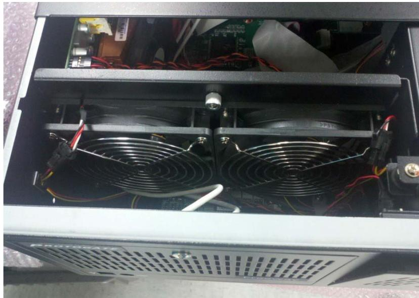
**Figure 2-3:** Fan Tray and Power Connectors
