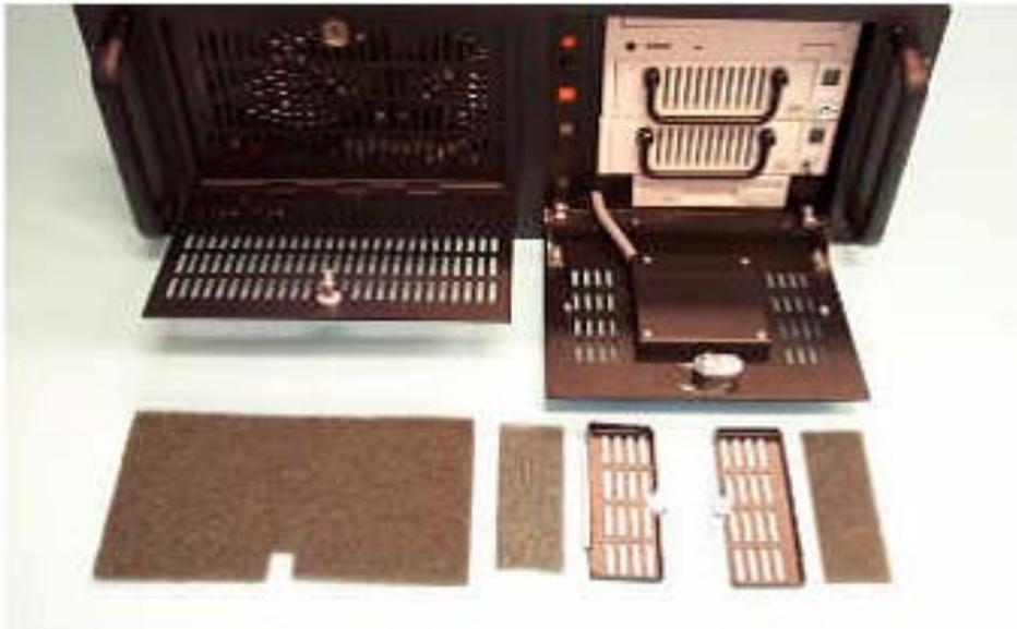
**Figure 2–6:** Fan Filters
