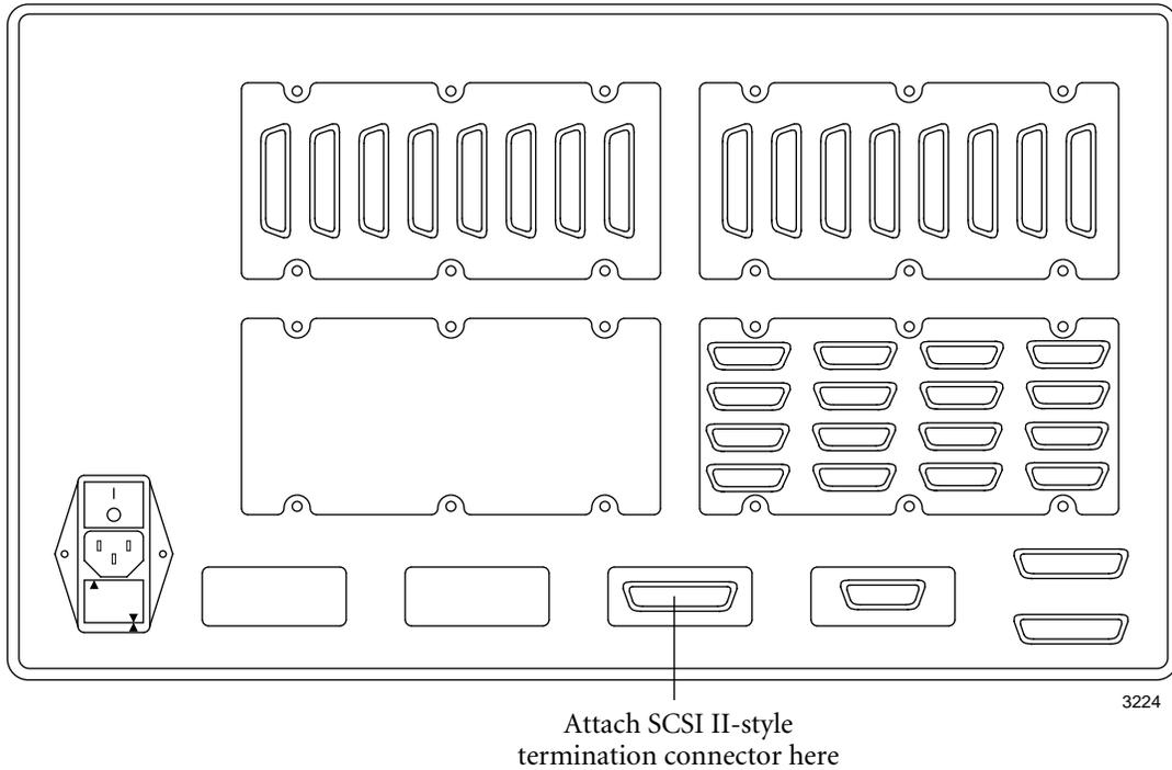
**Figure 2–8:** SCSI II-style Termination Connector Attachment
