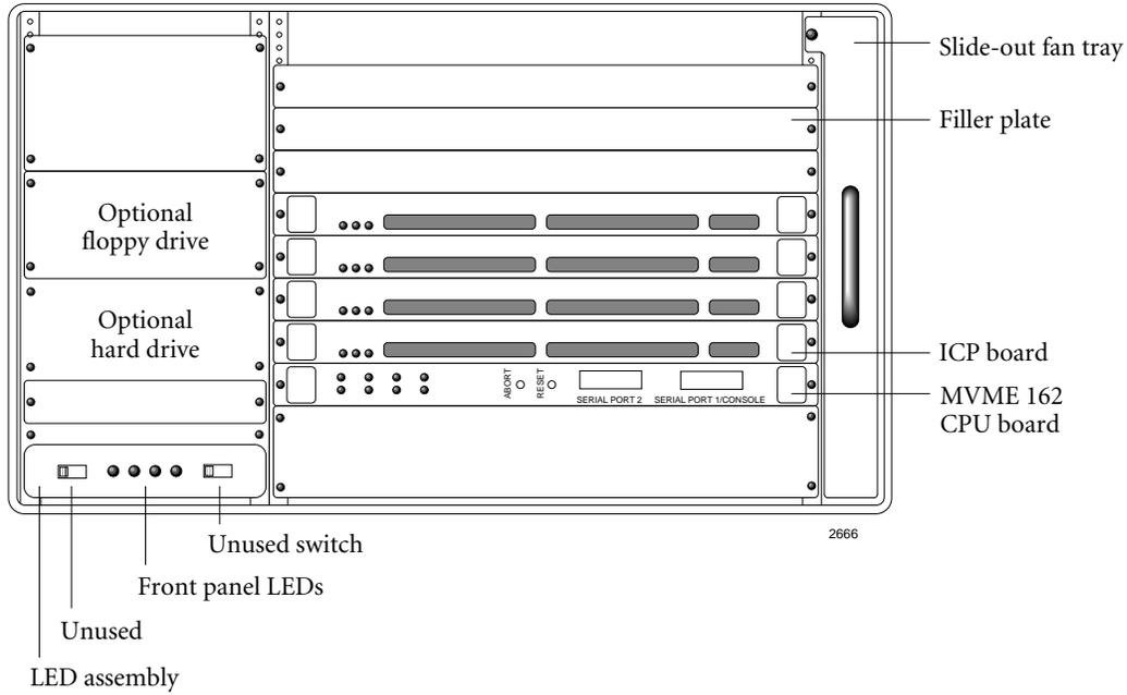
Figure 2-2: Front Panel: Freeway 4000 with MVME 162 CPU Board
