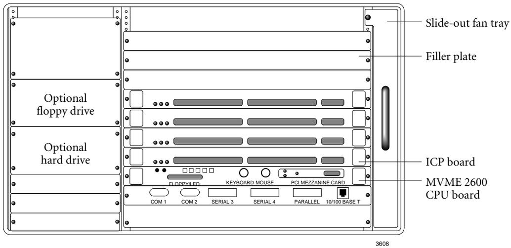
Figure 2-3: Front Panel: Freeway 4000 with MVME 2600 CPU Board
